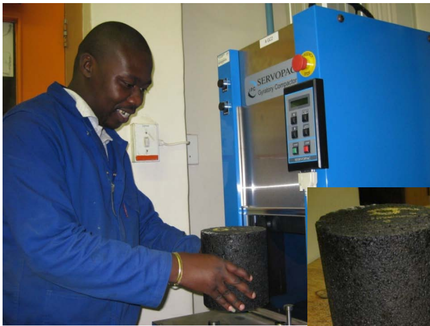
150 mm dia. x 170 mm GC specimen
