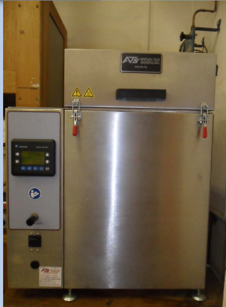
Pressure Aging Vessel for binder aging
