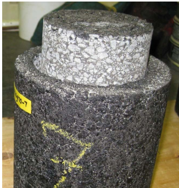
100 mm dia. X 170mm high cored from 150mm dia. X 170 mm high)
