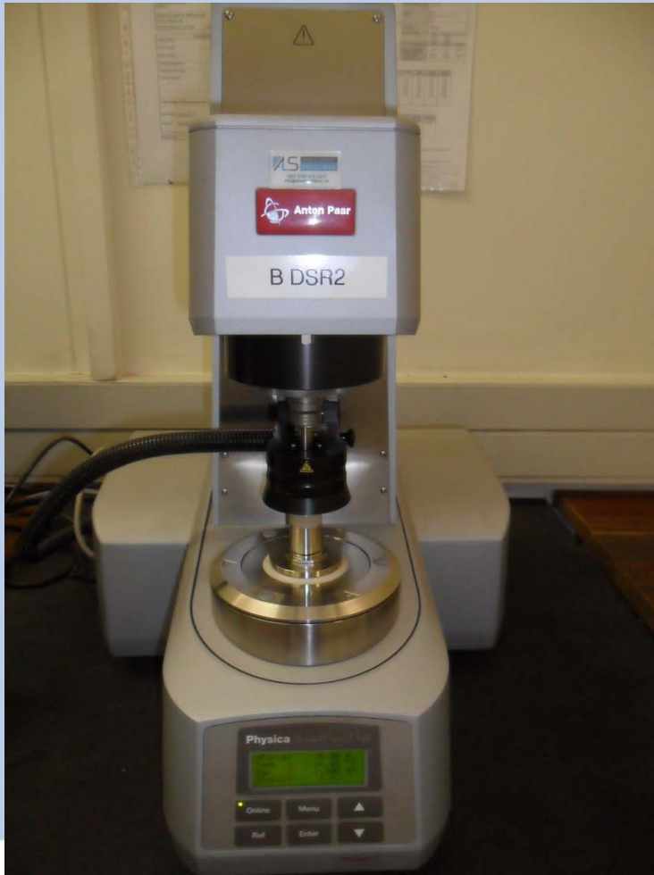
Dynamic Shear Rheometer for binder testing (R680k)
