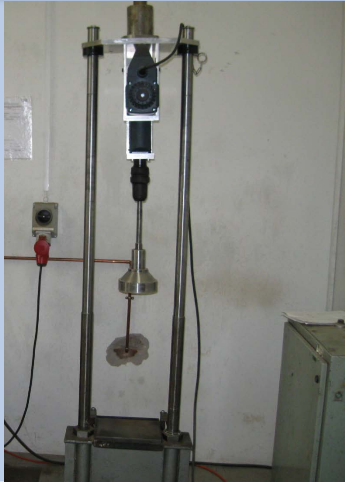
Vibratory hammer for compaction of materials
