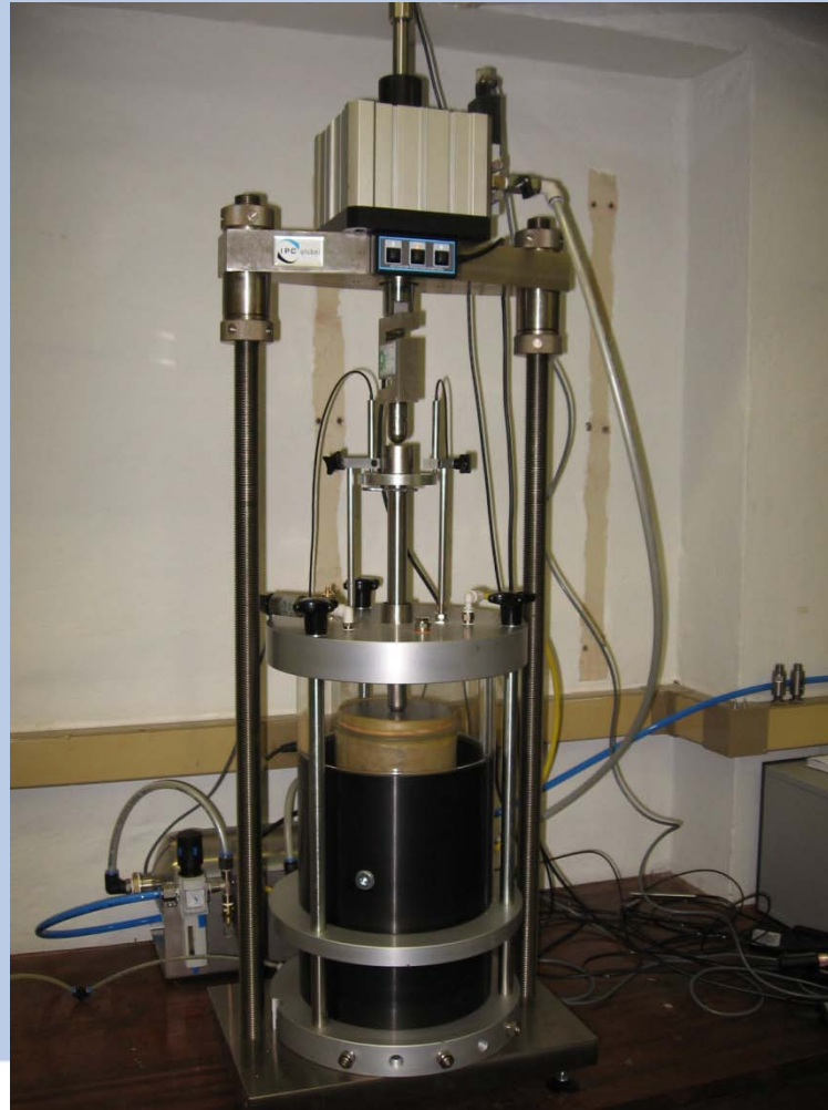
Triaxial machine for resilient modulus testing (R595k)
