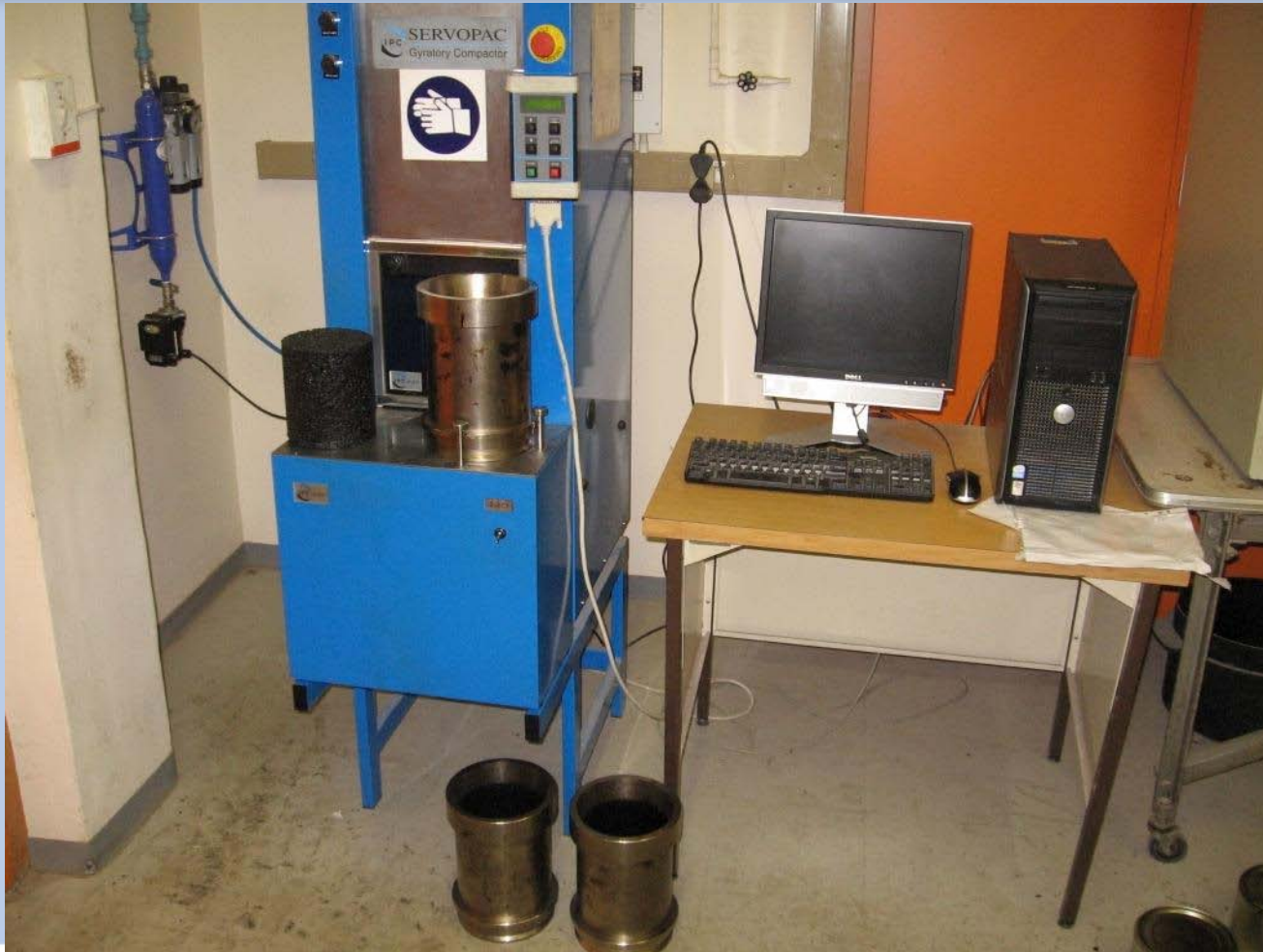
Advanced Asphalt Gyratory Compaction Equipment (R470k)
