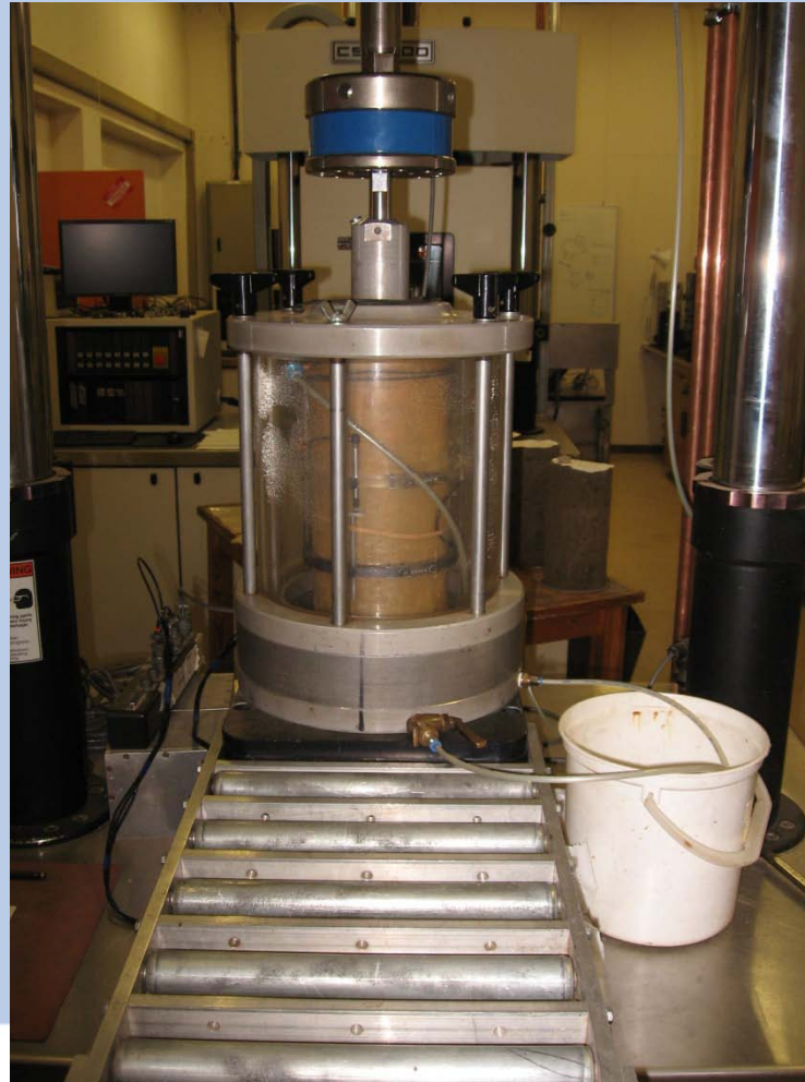
Triaxial Testing machine for resilient modulus testing
