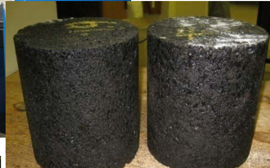
150 mm dia. x 170 mm GC specimen
