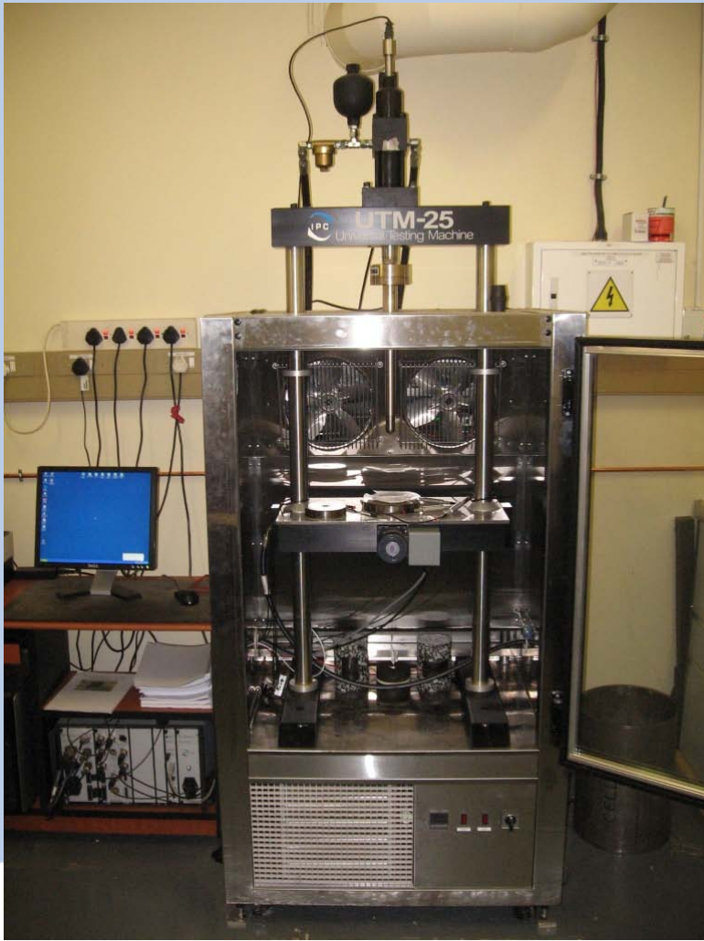
Dynamic modulus & Permanent Deformation Testing Equipment (R1.15m)
