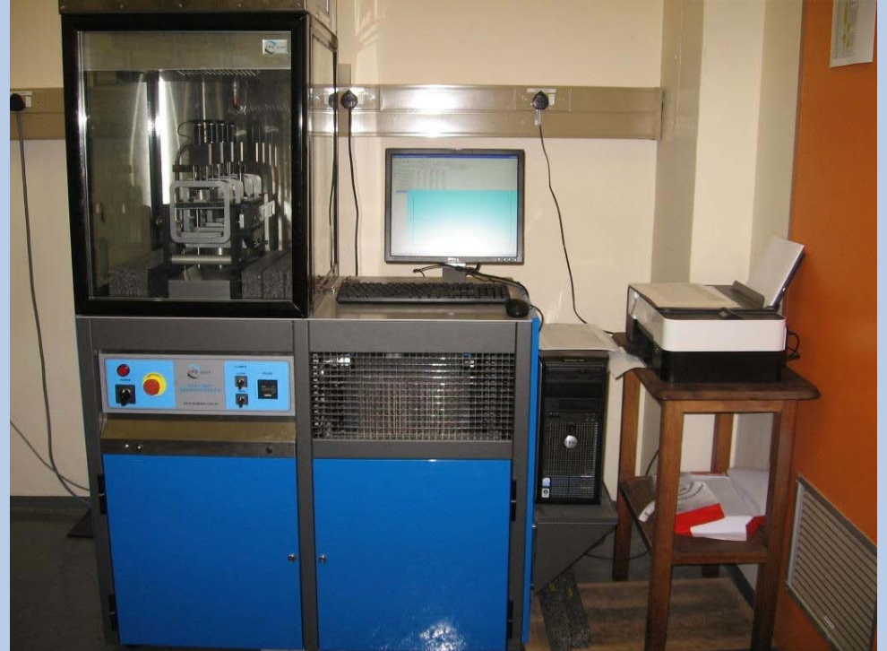
Beam Fatigue Testing Equipment (R900k)
