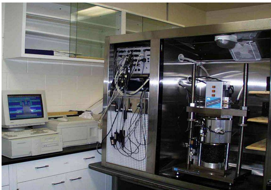
FIG. 3— RaTT Cell advanced triaxial test setup at ATREL.
