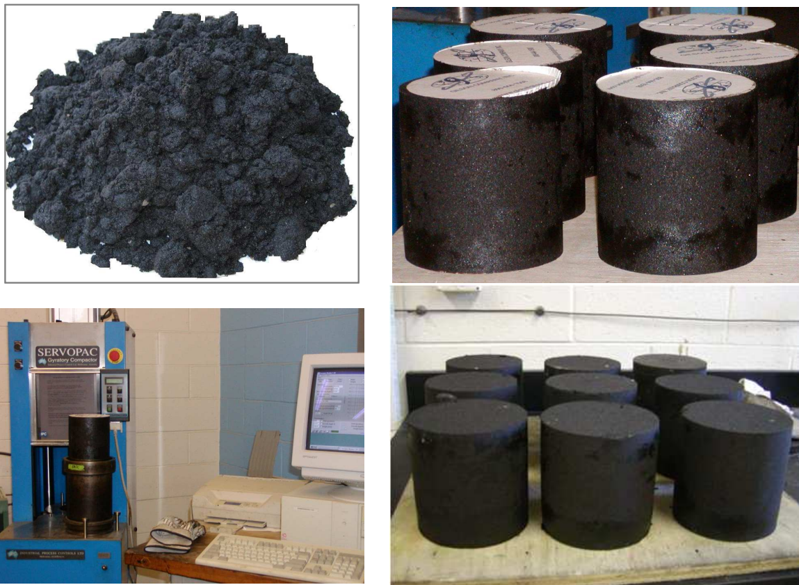
FIG. 1—Oil sand loose samples, samples prepared, and compaction equipment.
