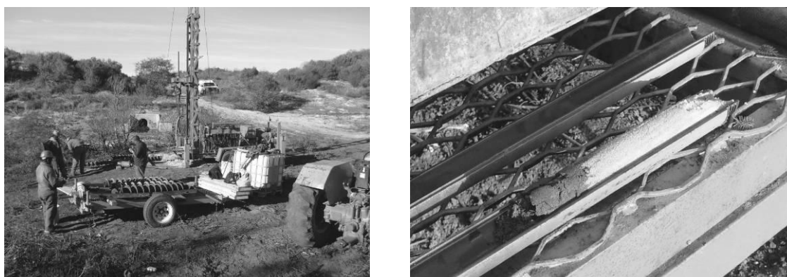
Figure 8.7: Auger drilling for unsaturated zone sampling in Basin #12; split spoon core (right)
