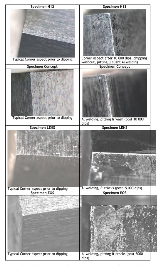
Figure 5: Optical micrographs of the specimen corners and notches at 5x magnification
