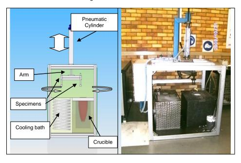
Figure 3: Aluminium Melt Cyclic Dipping Test Rig
