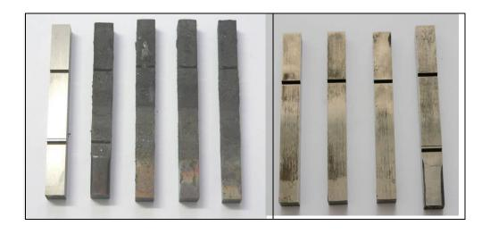
Figure 4: Specimens prior and after 10 000 Aluminium Melt Dipping Cycles
