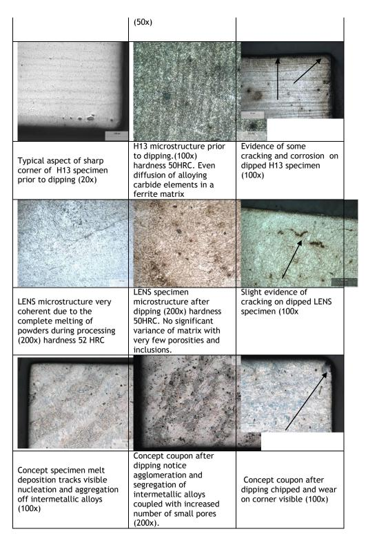
Figure 6: Optical micrographs of H13, LENS, Concept Laser and EOS samples
