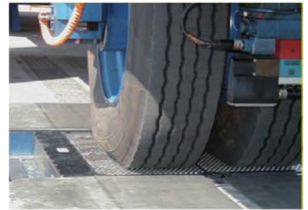
Figure 4: Dual SIM device under dual tire loading using the Heavy Vehicle Simulator (HVS) for testing
