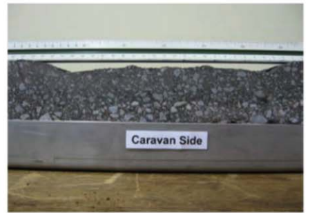
Figure 6b: This road sample displays rutting or plastic deformation in asphalt surfacing. Heavy Vehicle Simulator (HVS) tire (over) loading of 40 kN, and inflation pressure of 420kPa (with typical "m-shape" vertical stress distribution), resulting in typical "m-shape" plastic deformation in a thin asphalt surfacing layer – only one tire HVS traffic lane is shown here 23
