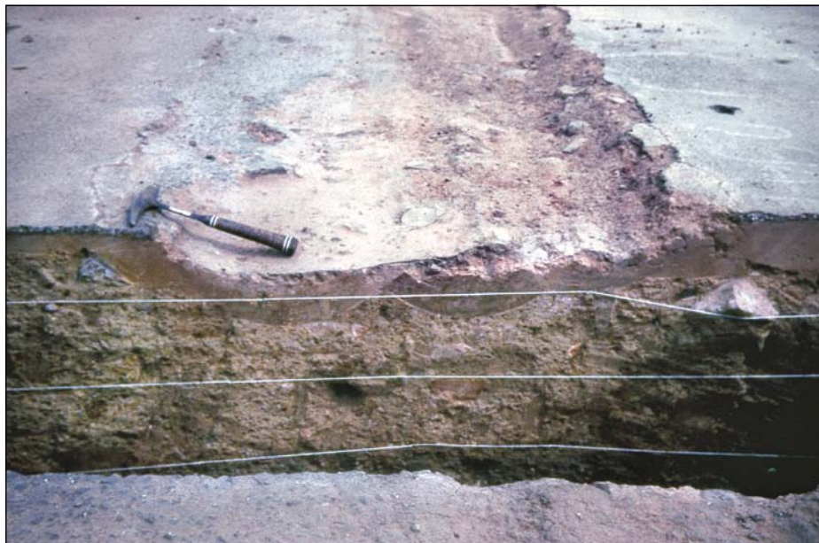
Photo 23 Final state of the lightly cemented base layer after HVS testing and crushing, in the wet state (De Beer 1990). Note the amount of material lost from the wheel path in centre of photo
