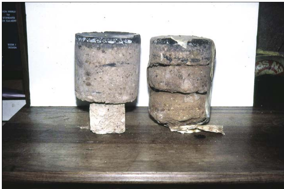
Photo 24 Field cores from lightly cemented base layer – left core: solid; right core: weak interlayers
