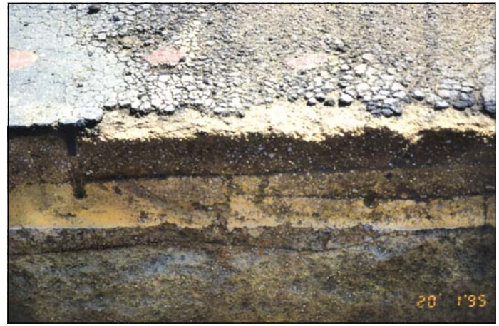
Photo 27 Crushing failure of the top of a lightly cemented base layer – final state of the lightly cemented base layer after some HVS testing
