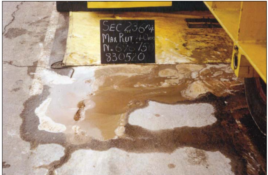
Photo 16 Fine material pumping from HVS test from Road P30 at Hornsnek in 1985 (Opperman 1984)
