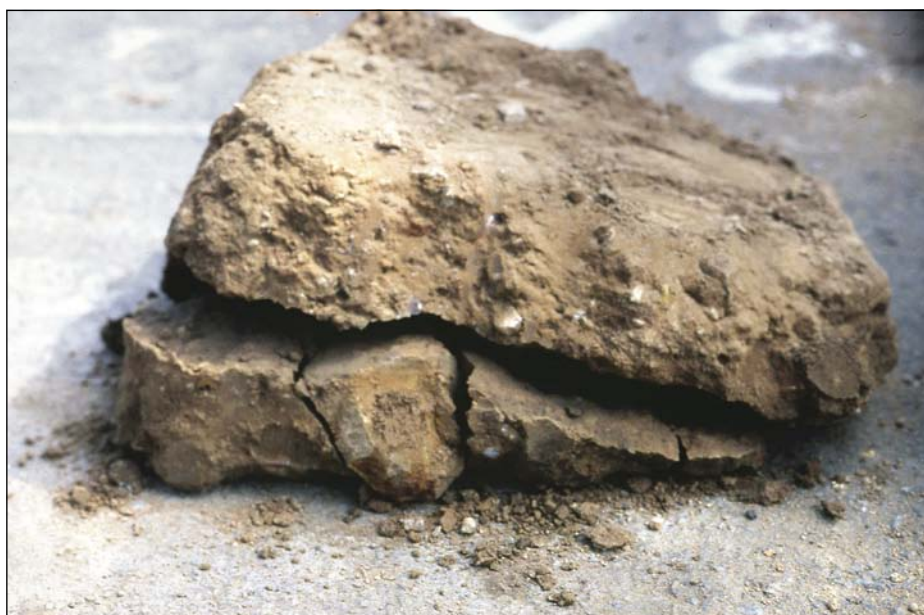
Photo 25 Signs of delamination (possible construction plane) in a lightly cemented layer (De Beer 1990)
