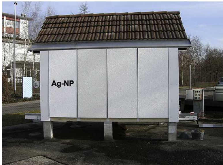
Model house with panels with the Ag-NP paint
