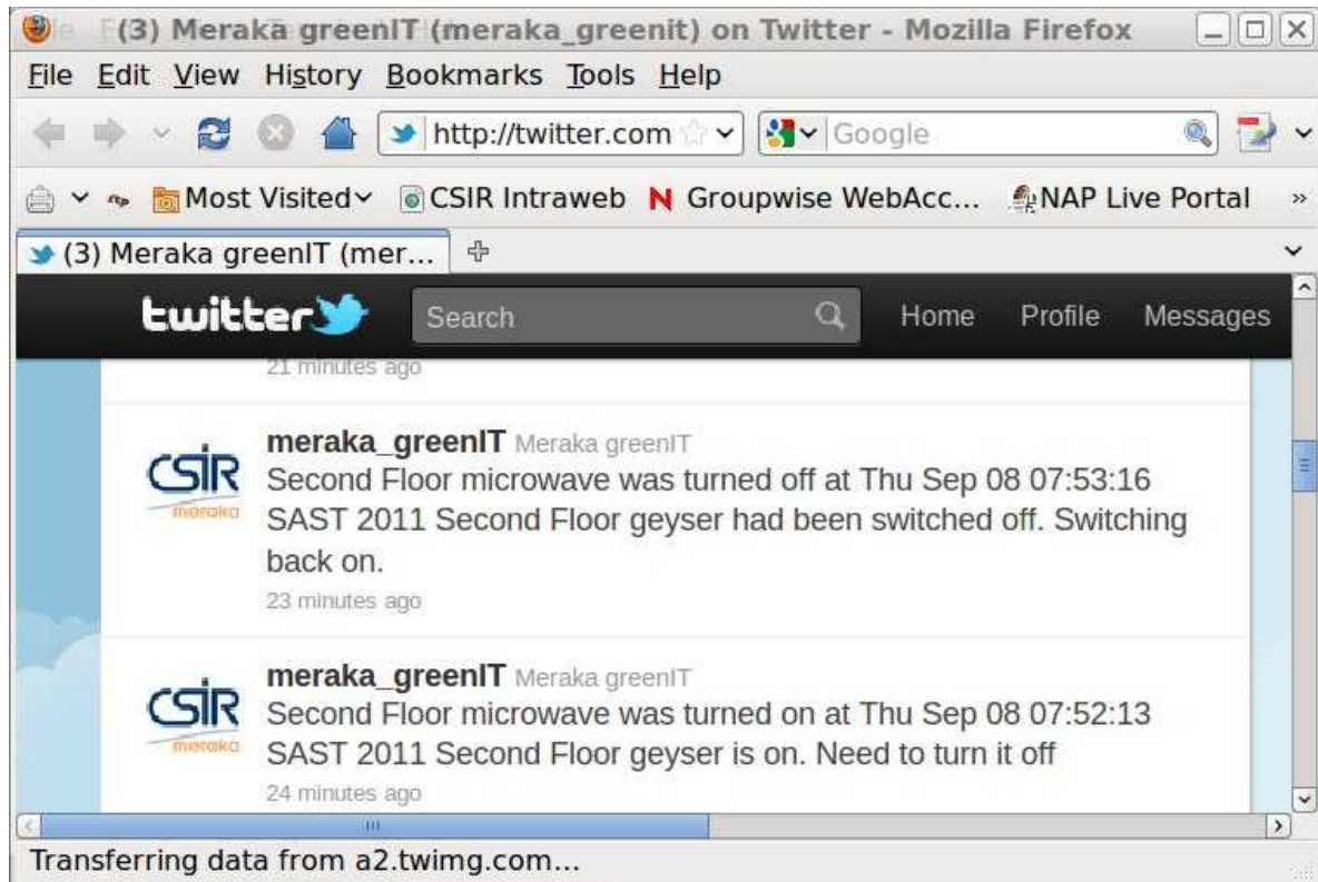
Illustration 3: Simple example of turning the geyser off then on again
