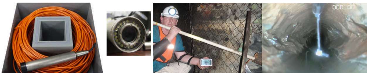
Figure 2 From left to right, a borehole camera (Raax SC-200, see Raax, 2008), a palmtop video recorder JXD990 and an example of the breakout images and a vertical marker in a BX hole
