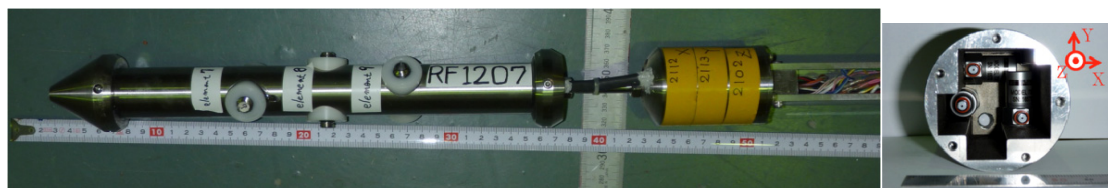
Figure 4 A sensor boat to monitor dynamic stress change (left; fast responding, high-capacity strain gauges) and fault displacement with X-, Y-, and Z component accelerometers at rupture front (Watanabe, 2010)
