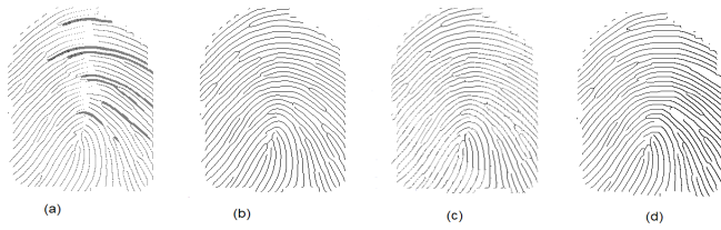
Fig. 11. (a) Skeleton produced by Abdulla et al's algorithm from image 1; (b) Skeleton produced by Guo-Hall's algorithm from image 1; (c) Skeleton produced by Hall's algorithm from image 1; (d) Skeleton produced by Zhang-Suen's algorithm from image 1
