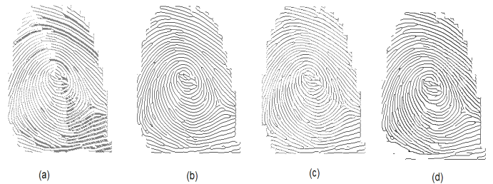
Fig. 14. (a) Skeleton produced by Abdulla et al's algorithm from image 4; (b) Skeleton produced by Guo-Hall's algorithm from image 4; (c) Skeleton produced by Hall's algorithm from image 4; (d) Skeleton produced by Zhang-Suen's algorithm from image 4
