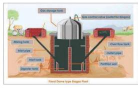
Biogas digesters can process different feedstocks, and be implemented in a variety of applications, including:
