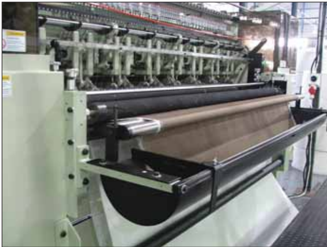
CNC mediated material slitting with backing and stitching also being added to allow for capping that is added to the side of the mattress
