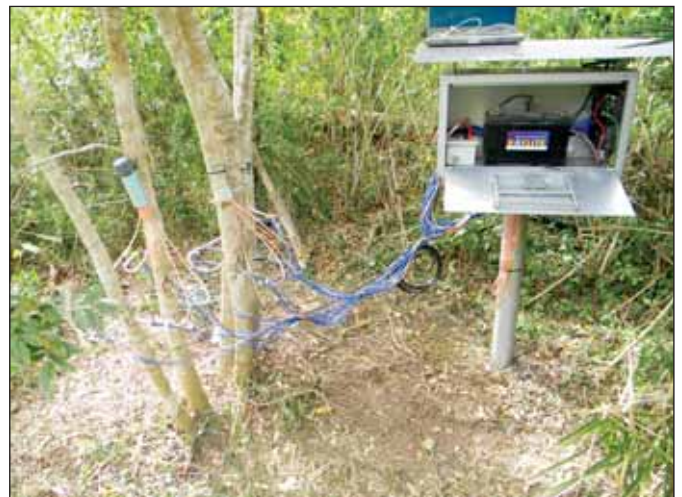
Figure 2: Heat Pulse Velocity system for measuring hourly sap flow rates, and resultant water-use volumes, in individual tree stems. (Photo: M Gush)
