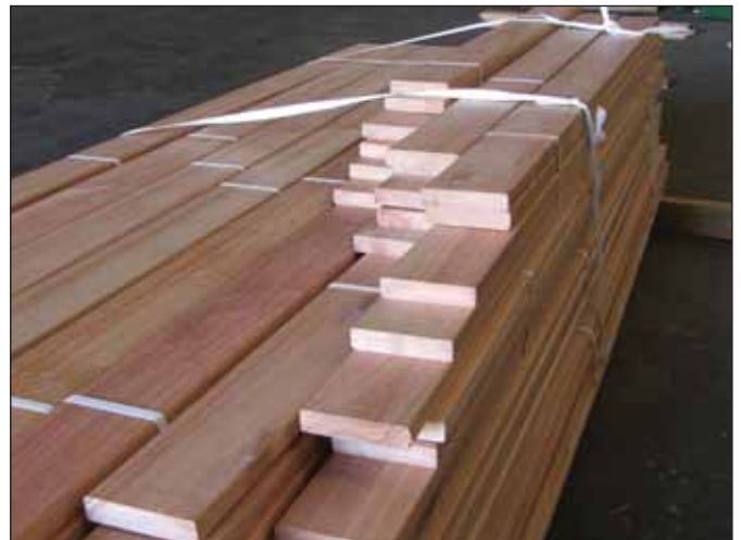
Karri decking exiting Profile Timbers' Alberton-based production site
