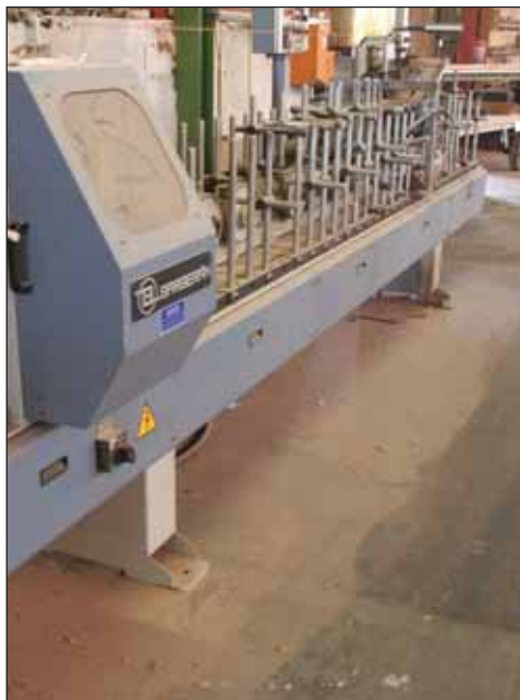
Two Barberan profile wrap platforms provide for Profile Timbers' foil upgrading capacity
