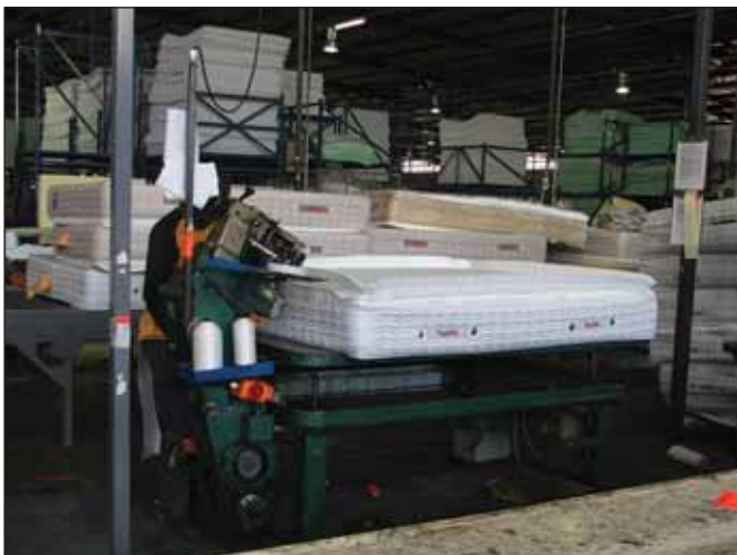
Piping going onto the almost complete mattress
