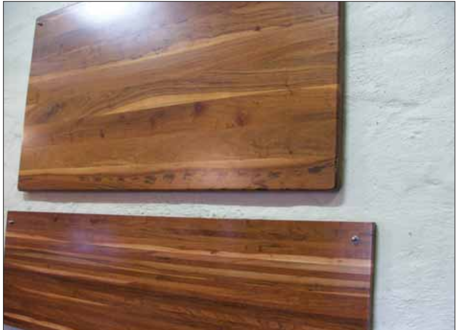
Tongue and groove flooring with sapwood adding further variation to heartwood grains
