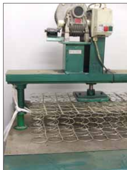
BSPG testing facility where bedding products are tested to ensure compliancy with international standards
