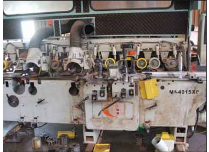
Part of Profile Timbers' moulding capacity, a IWM five-head moulder supplied by GF Potgieter Woodworking Machinery
