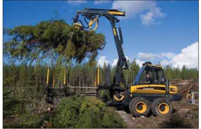
Ponsse's BuffaloDual + EH25 harvesting head doing energy harvesting service. Note the slash containing top half of the tree being loaded with the need for bundling therefore becoming obsolete
