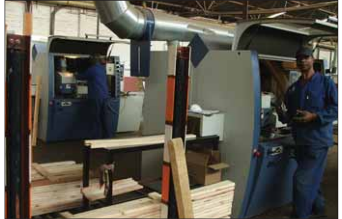
Five Weinig Unimat 500 moulders form the backbone of BSPG's base manufacturing division
