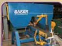
Baker horizontal band resaw, 11kW including blade setter/sharpener
