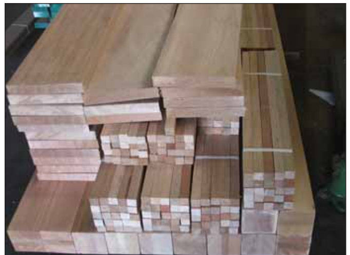
A complete decking order awaiting collection. Note the laminated balustrading, that again resulting from Allan Day's stay at RSB is laminated with Kleibert PUR 501 adhesive, sourced from A Huster Machine Tool Company
