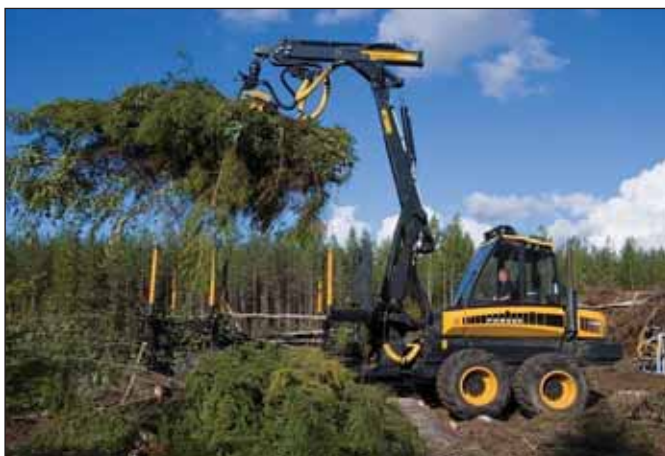
Ponsse's focus is on mechanised platforms that can migrate from normal harvesting to energy harvesting without the need for major adaptations
