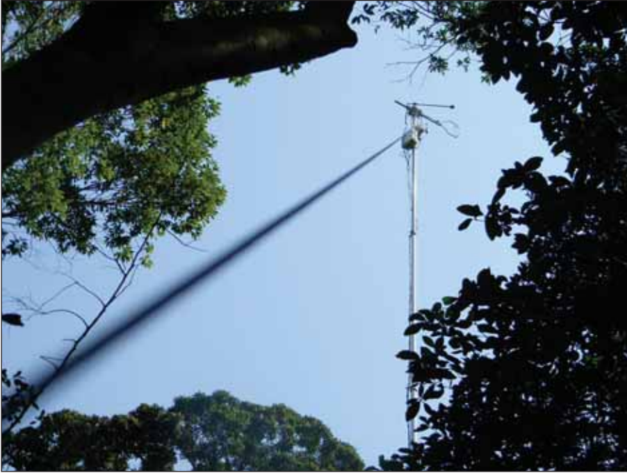
Figure 3: CSAT Eddy Covariance system, mounted on a telescopic mast, for measuring total evaporation (water-use) above the canopy of an indigenous forest (Photo: M Gush)
