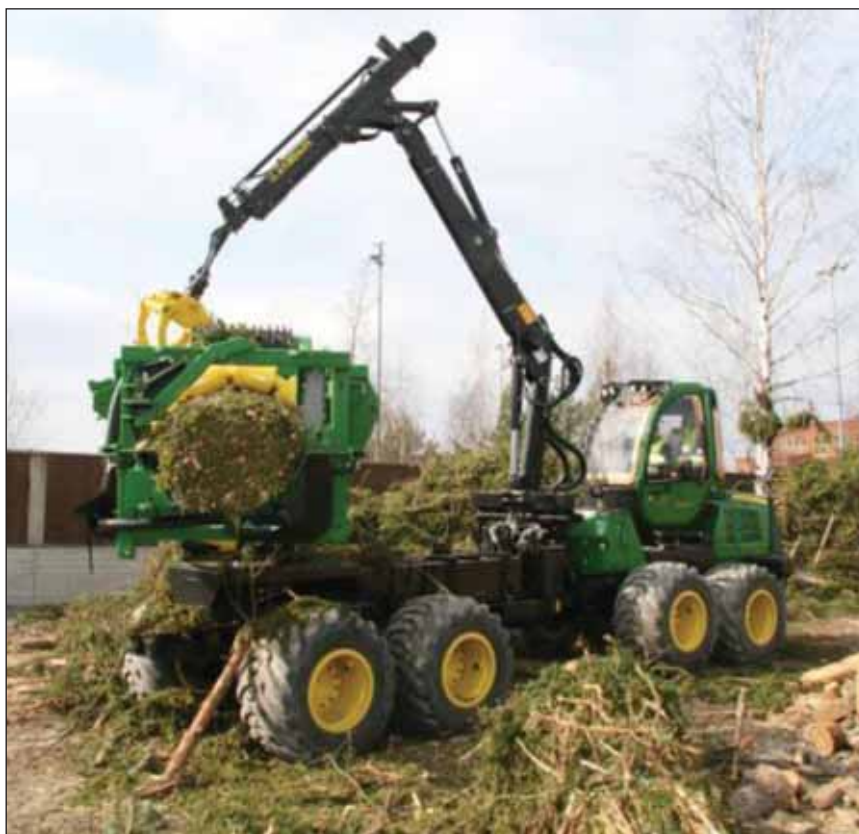
The John Deere JD1190E slash bundler in action
