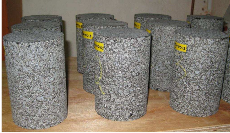
Fig. 1. Cylindrical 100 mm diameter by 150 mm high specimens.
