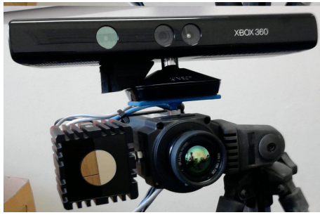
Fig. 1. Capture Setup: Microsoft Kinect (top); Mesa SR4000 (left); FLIR A300 (right).
