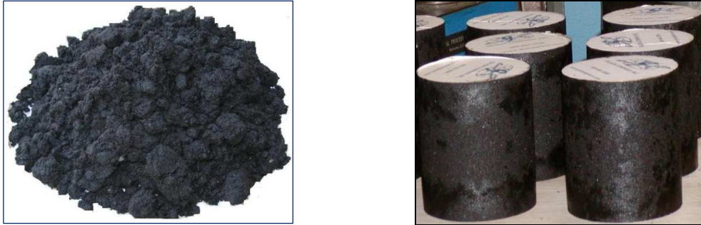
(a) AU-14 Oil sand sample in natural state; (b) Gyratory compacted AU-14 specimens
