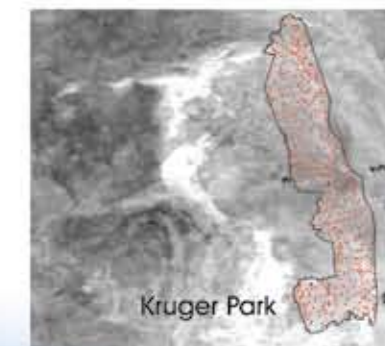
1 km AVHRR growth season sum (ΣNDVI), 533 fixed field sites for long-term monitoring in KNP
