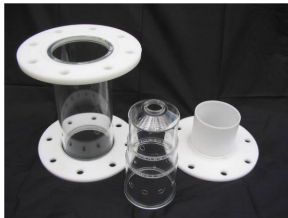
Figure 3: The transparent combustor parts - casing, liner and outlet pipe
