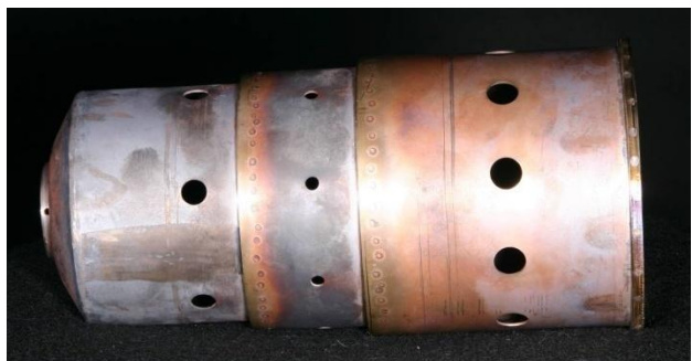
Figure 2: The metal combustor liner
