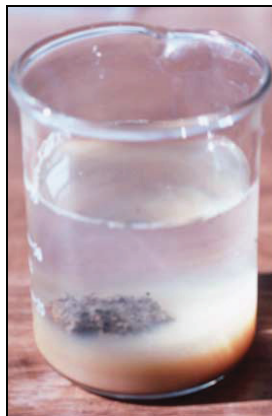
Figure 3: Colloidal suspension of a highly dispersive soil- Grade: 4- strong reaction
