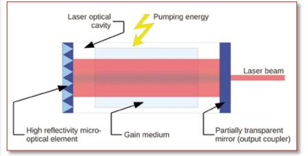
A schematic of a laser, showing the three core components: the resonator bound by the two end mirrors, a gain medium, and a means to excite the gain medium.
