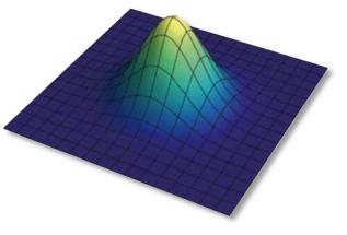
A Gaussian profile laser beam, with a characteristic peak at the centre and slow decay at the edges.
