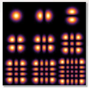
When the laser operates in rectangular symmetry, the output light patterns (called modes) form 2D patterns of light following what are called Hermite–Gaussian functions. The number of null lines between the 'spots' of light correspond to the order of the functions – more spots, higher order.
