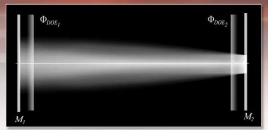
The resonator concept, as shown here, comprises two transparent DOEs (like lenses) at either end as well as the usual bounding mirrors to complete the box.
