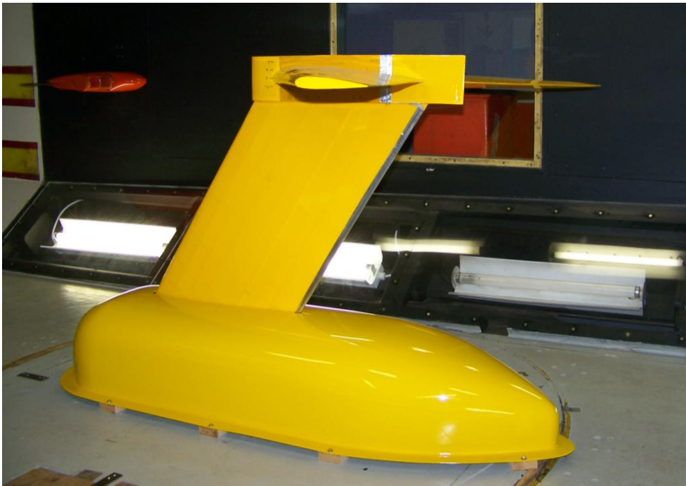
Fig. 3: T-tail model installation in the wind-tunnel
