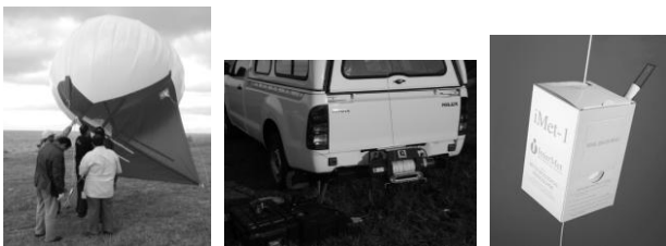
Figure 8. Photograph of the 11 cu m Skyhook Helikite (left), Winch setup (centre) and iMet-2-AB radiosonde (right).
