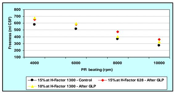
Figure 6: Freeness vs. beating relationships for the control and GLP+ KP under different Kraft pulping stage pulping conditions
