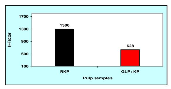
Figure 2: Comparison between regular Kraft pulping (RKP) and green liquor pre-treatment modified Kraft pulping (GLP+KP) on H-Factor required to produce pulp samples at a target Kappa number. Note RKP was performed using 15% liquor change, 170°C at H-Factor of 1300. While the GLP+KP was conducted using 15% liquor change, 170°C and the H-Factor was varied in the Kraft pulping stage until the target Kappa same as in RKP was obtained
