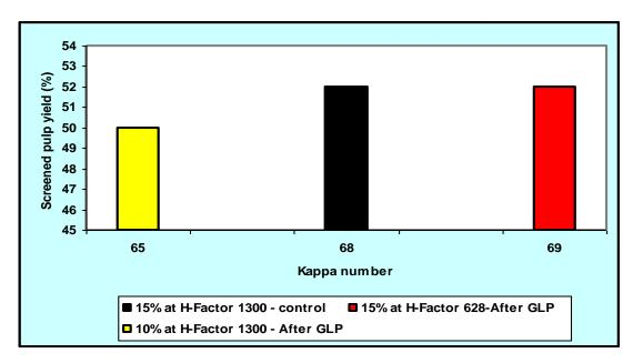
Figure 5: Illustration of Kappa number and the corresponding screened pulp yield (SPY) obtained for the control and GLP+ KP under different Kraft pulping stage conditions
