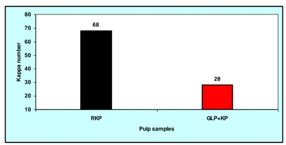
Figure 1: Comparison between regular Kraft pulping (RKP) and green liquor pre-treatment modified Kraft pulping (GLP+KP). Note RKP pulp samples were produced using regular Kraft pulping method using 15% liquor change, 170°C at H-Factor of 1300. While the GLP+KP pulp samples were produced after GLP followed up with regular Kraft pulping method using 15% liquor change, 170°C at H-Factor of 1300
