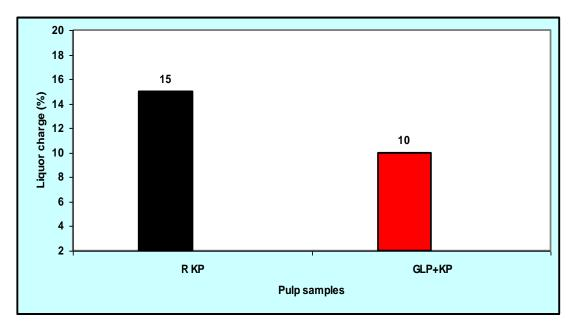
Figure 3: Comparison between regular Kraft pulping (RKP) and green liquor pre-treatment modified Kraft pulping (GLP+KP) on liquor charge required to produce pulp samples at a target Kappa number. Note RKP was performed using 15% liquor change, 170°C at H-Factor of 1300. While the GLP+KP was conducted using H-Factor of 1300 at 170°C and the liquor charge was varied in the Kraft pulping stage until the target Kappa same as in RKP was obtained
