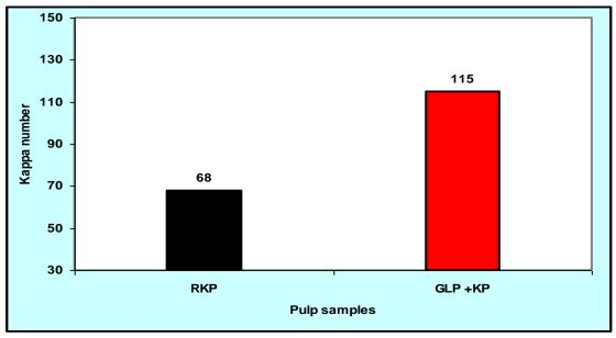
Figure 4: Effect of reducing both liquor charge and H-Factor on Kappa number in GLP +KP. Note RKP was performed using 15% liquor change, 170°C at H-Factor of 1300 . While the GLP+KP was conducted using 10%, 170°C at H-Factor of 628
