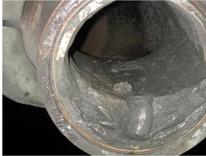
Figure 2: Cemented Paste Fill Deposit under Laminar Flow Conditions
