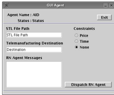
Figure 4: The GUI agent interface described here provides a pop up screen presented by the agent to its human controller. The purpose being that the agent wishes to obtain additional information relating to the rapid prototyping process and what CAD file to be produced.
