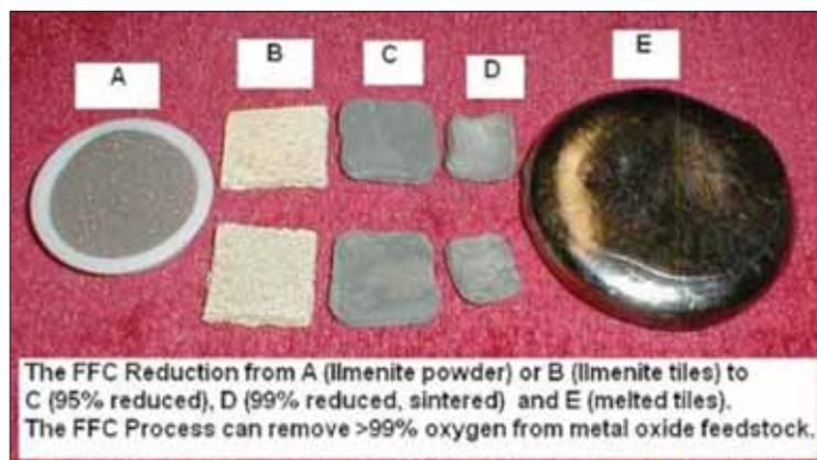
Figure 1—FFC process: from mineral to metal
