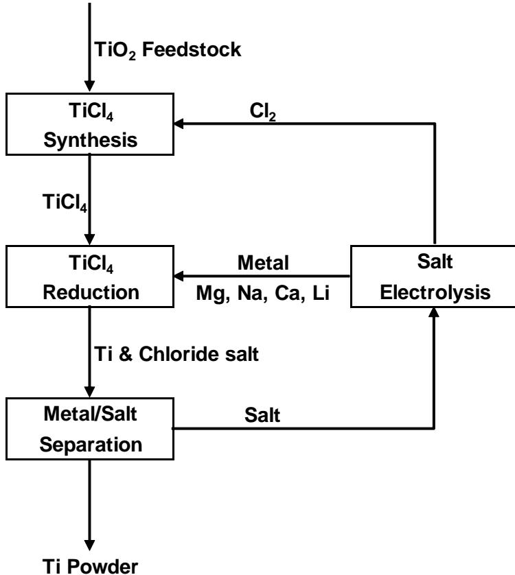
M.P. of salt determines reactor temperature, construction materials & heat exchanger design.
