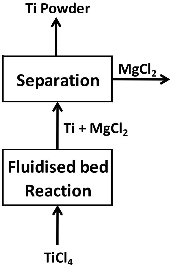
$$T_{\text{M.P.Mg}} < T_{\text{reactor}} < T_{\text{M.P.MgCl}_2}$$
