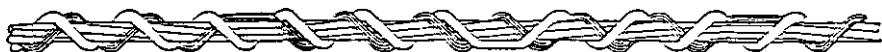
Fig. 2 - Second continuous filament wrapped around the first, out of step by half of one twist zone 11 .
