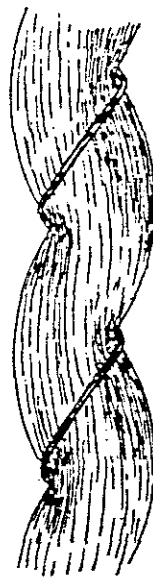
Fig. 17 - Wrap yarn spun with too high filament tension 65 .
