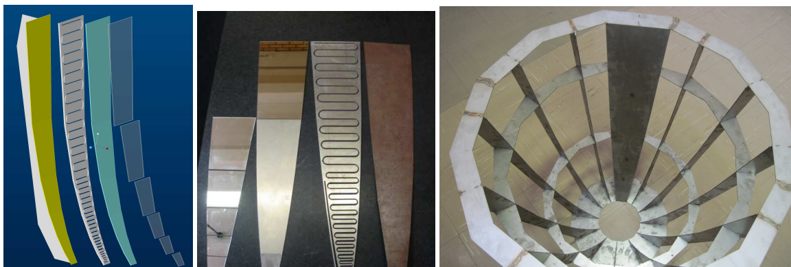
Fig. 3. Left: conceptual layout; Centre: mirror facets, thermal spreader plate, cooling plate and backing plate; Right: ribs welded into frame with 1 backing plate
