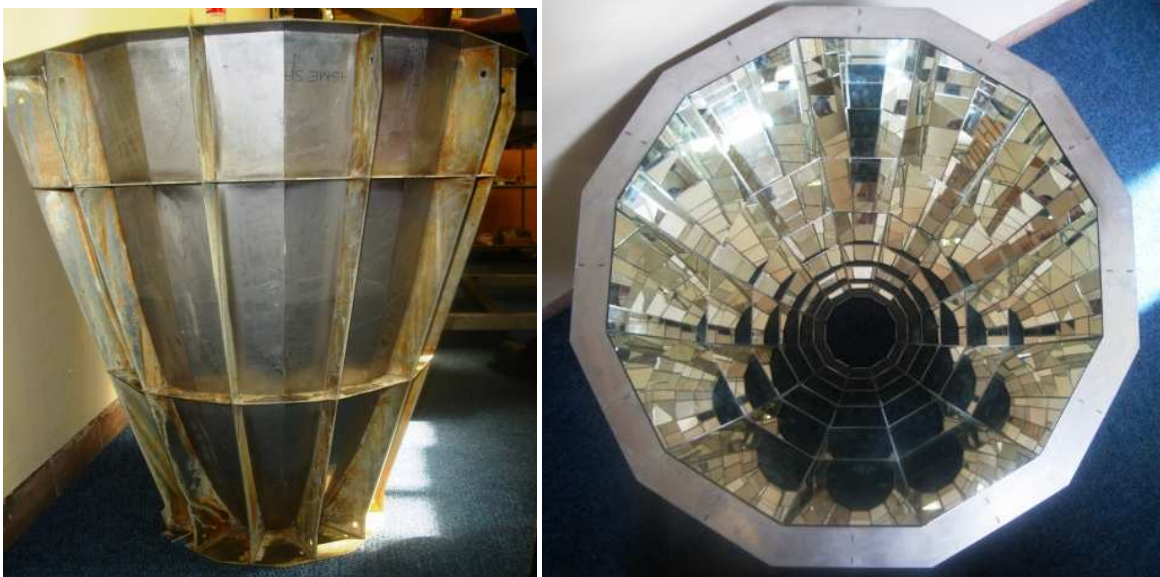
Fig. 4. Left: Complete frame and backing plates, Right: CPC view from above with all mirror facets temporarily in place
