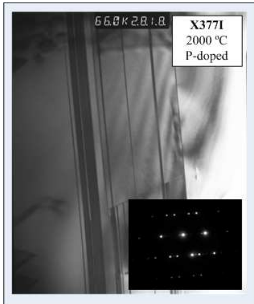
Fig. 9: Bright Field TEM micrograph and SAD of sample X377I after annealing at a temperature of 2000°C. The SAD indicates that a phase transformation to 6H-SiC hexagonal phase occurred. The beam is along the \langle 100 \rangle .
