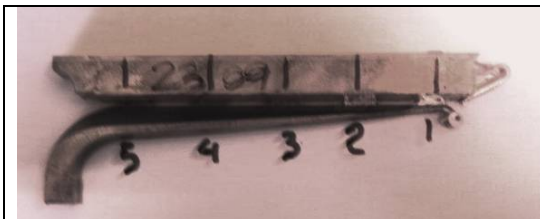
Figure 17: Specimens cut from feeding tree of standard runner through the 5 gates
