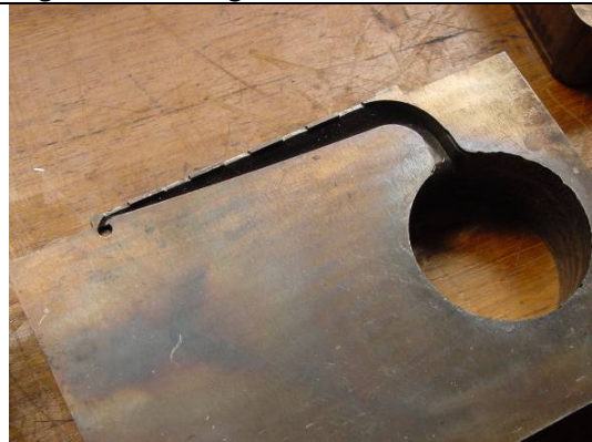
Figure 9. H13 feeding area insert after producing 5 000 shots
