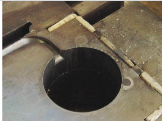
Figure 10. Anviloy 1150 feeding area insert After producing 5 000 shots
