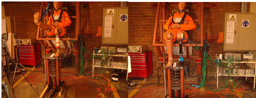
Figure 7: Hybrid III ATD with SA leg (left) and THOR-Lx leg (right).
