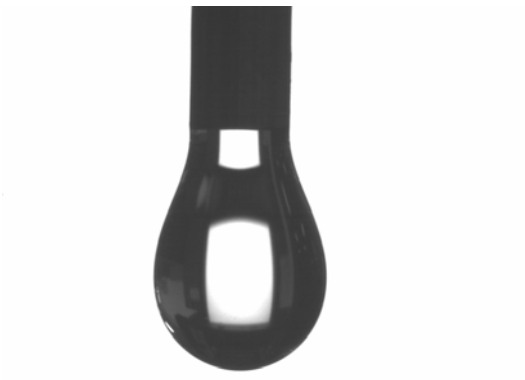
Fig. 3 (b): Pendant drop from a 50mg/ml solution of BSA. The droplet has attached less on the needle due to the fact that the surface tension has decreased. This causes the droplet to fall off easily from the needle.
