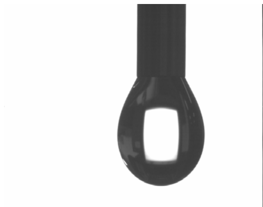
Fig. 3 (a): Water pendant drop, hanging from a needle during surface tension measurements. The droplet has attached more on the needle because the surface tension is very high.
