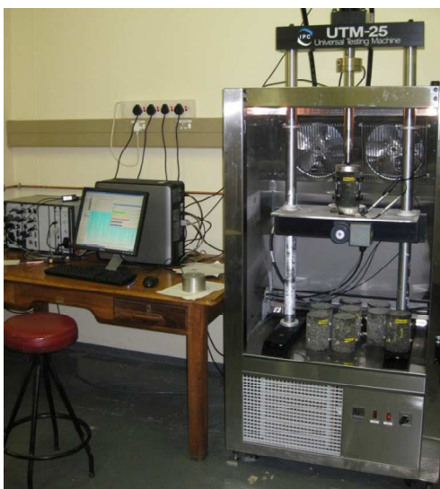
(a) Dynamic modulus specimens
