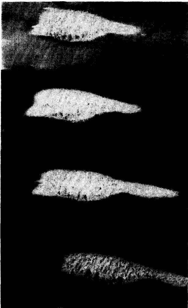
Fig 6 Type 1200 Al alloy samples eroded for 1 hour at 44.8; 49.8; 65.5 and 78.8°C from top to bottom. The inducer holes were located on the left
