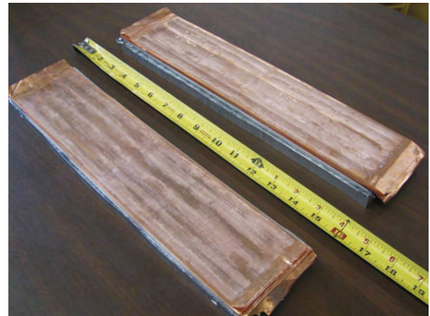
Fig. 2. Frontal view of an FGM sample made using a UC machine.
