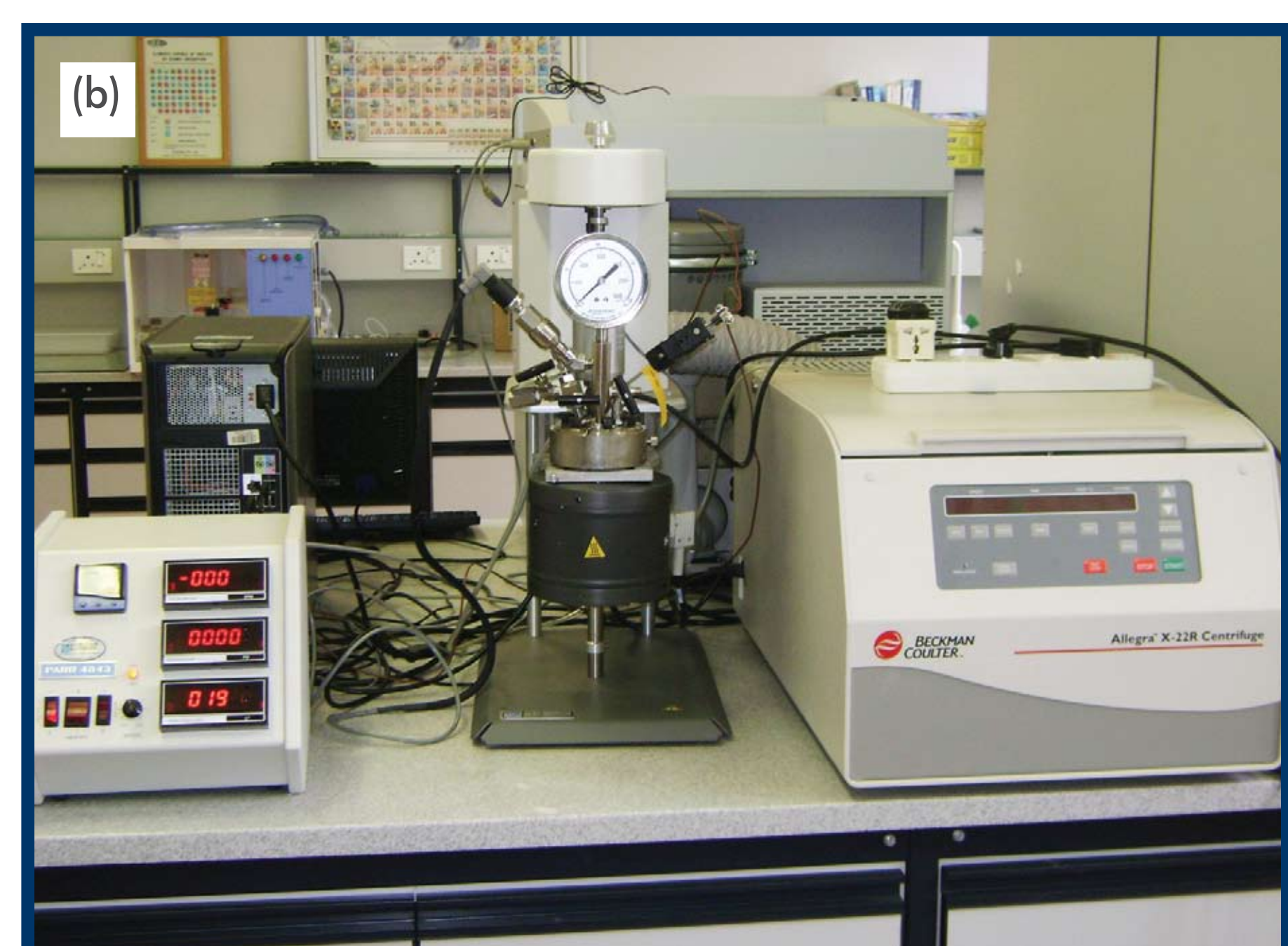
Figure 1: (a) High pressure system (autoclave) and (b) Microwave reactor unit for the synthesis of titania nanotubes (TNT) in a hydrothermal process
