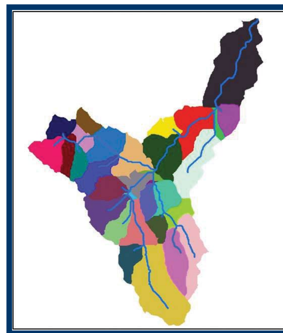
Figure 3: Example of spatial HRU delineation in the Sandspruit pilot catchment (150 km 2 )
