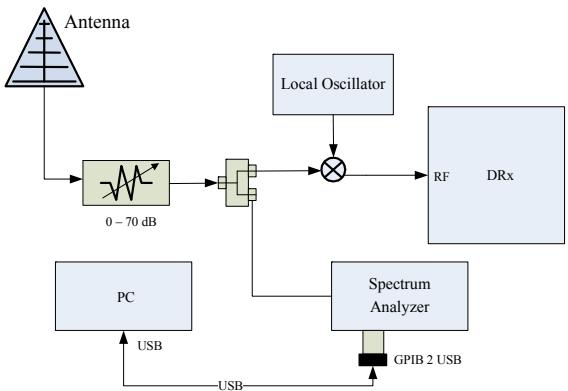
Figure 1. Setup for radar signal measurements
