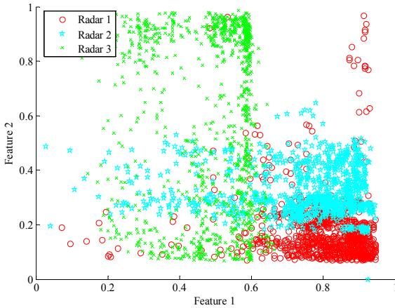
Figure 4. Clustering of two features for three different radars of the same system
