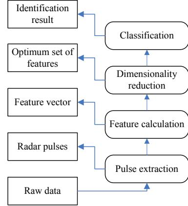
Figure 2. Specific emitter identification process
