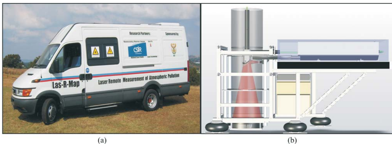
Fig. 1. (a) The mobile LIDAR van. (b) A pictorial representation of the LIDAR setup inside the van.
