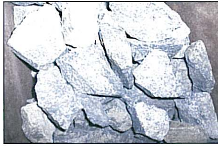
Figure 2 Example of crushed "hard" dolerite rock
