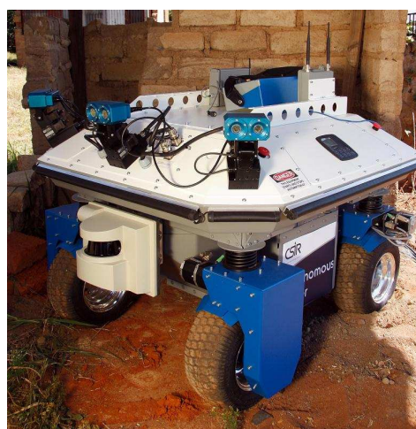
Fig. 1. The Seekur platform from Mobile Robots that the proposed controller was implemented on.
