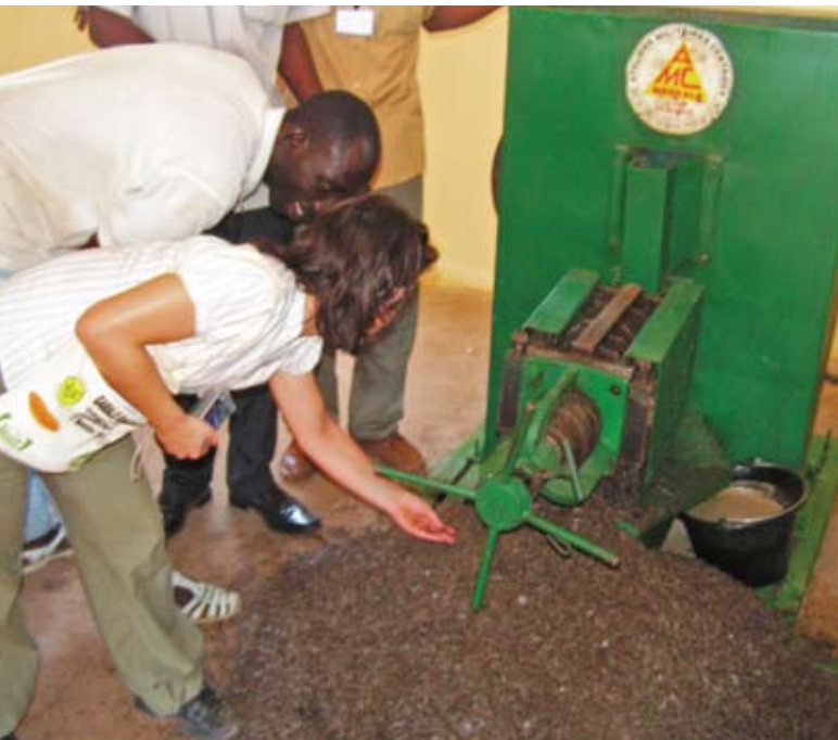
Extracting jatropha oil using a mechanical screw press at Mali Folkecenter, Garalo (Photo by Graham von Maltitz)
