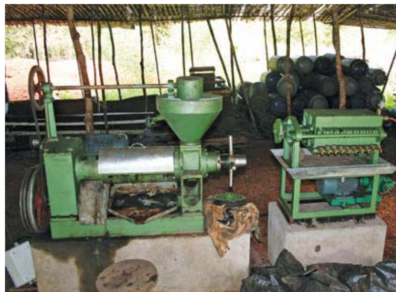
A small screw press for extracting jatropha oil stands idle due to low jatropha yields in a project just outside of Gorongosa Game Reserve, Mozambique (Photo Kevin Setzkorn)
