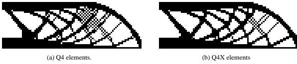
Fig. 5 Optimal topologies of the MBB beam using symmetry and employing (a) Q4 and (b) Q4X elements.
