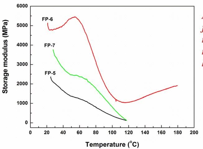
At 0.6 weight fraction of the matrix storage modulus was highest.
