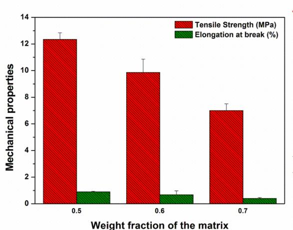
Increase in weight fraction of the matrix resulted in decrease in tensile strength as well as percentage elongation at break.
