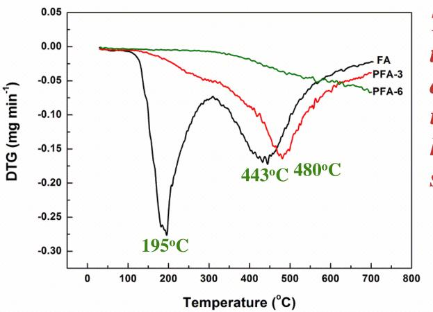
T<sub>max</sub> at lower temperature is absent in PFA indicating higher thermal stability of PFA.
