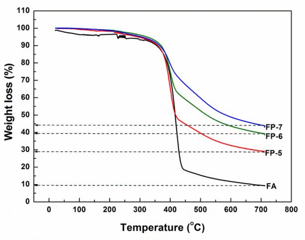
The increase in weight fraction of the matrix increased the thermal stability with higher charyield.
