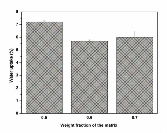
Water uptake of the composite was lowest at 0.6 weight fraction of the matrix which indirectly higher states water resistance. PLA based nowoven flax fiber at 0.7 weight fraction of matrix has water uptake of 9.8 %.
