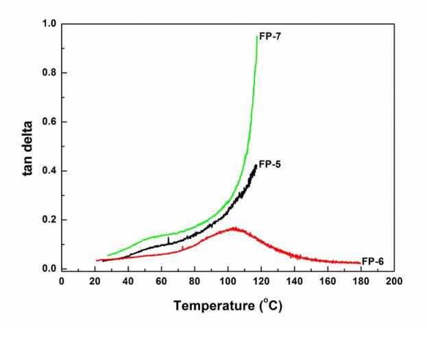
The lower damping factor at 0.6 weight fraction of the matrix indicates good compatability of matrix with fibers.
