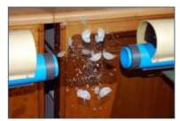
The hail gun releasing hail stones, targeted to hit the heliostat mirror nanel
