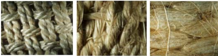
Figure 9. Weaving architectures of three types of sisal fabrics [25].
