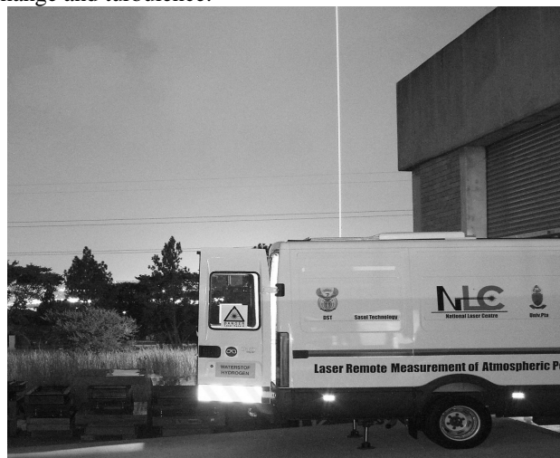
Figure 1: CSIR-NLC-Mobile LIDAR system
