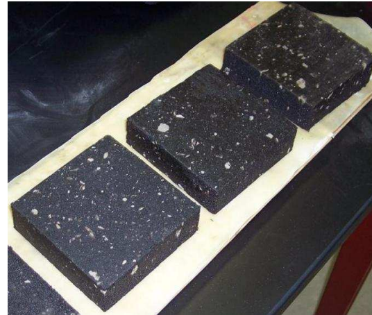
(b) Square prismatic direct shear test specimens
