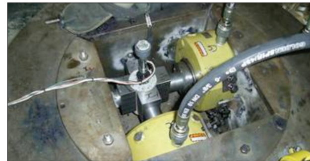
Figure 9—Mechanical biaxial test apparatus for doorstoppers
