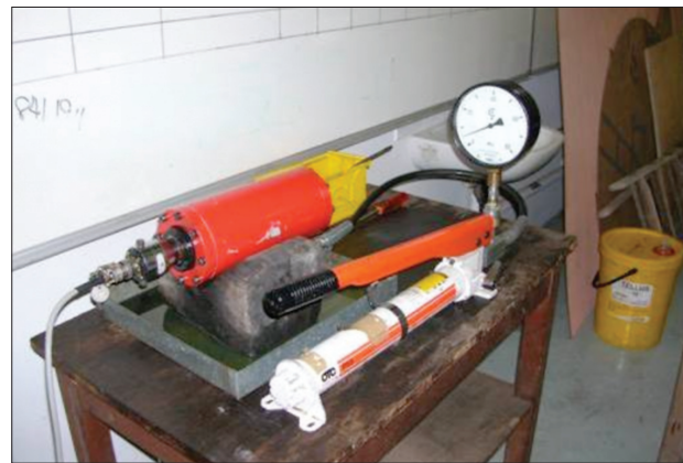
Figure 11—Test apparatus for loading triaxial cells
