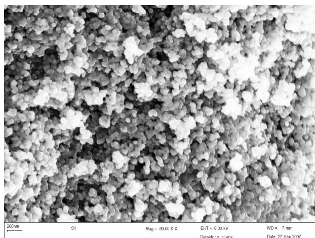
Figure 1. SEM image of untreated TiO 2 (P25-Degussa)
